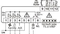
compressor relay is 8(3)A or 16(6)A according to the model.
