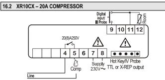
12Vac/dc supply: connect to the terminals 7 and 8. 24Vac/dc supply: connect to the terminals 7 and 8. 120Vac supply: connect to the terminals 7 and 8.
