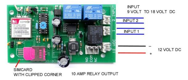
1: Slide the simcard in to the door making sure that the clipped corner of the simcard lines up with the clipped corner of the simcard holder.
